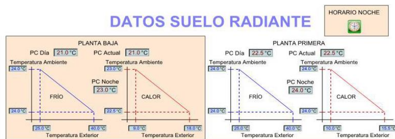
Fig. 2: Apolonio Morales 29, Madrid. Control System interface. Radiant floor Setpoint Manager. Source: Apolonio Morales 29, Madrid, Control System.
